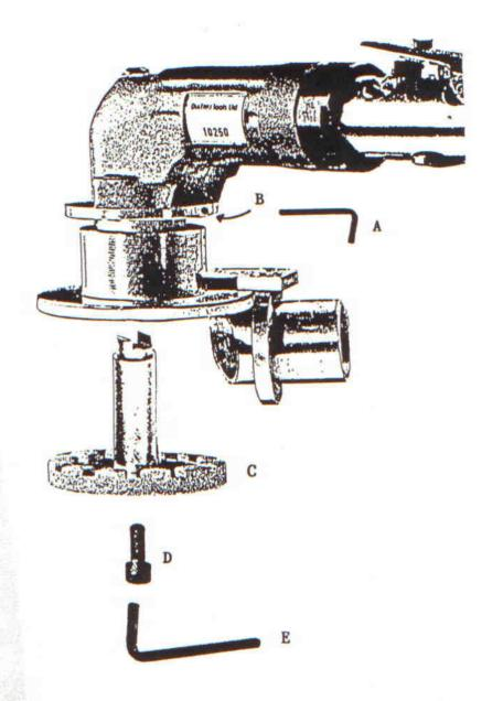
Insert 1/8 Allan key (A) into pin hole (B) to lock flange from turning. Insert cutter (C) into tool flange and turn slightly until cutter locks into flange and will not turn. Insert locking bolt (D) into end of cutter and push all the way down to end of cutter until bolt reaches flange. Using 1/4 Allan key (E) tighter bolt clockwise. This bolt locks cutter into tool. Remove 1/8 Allan key. Spin cutter by hand to check if secure.
